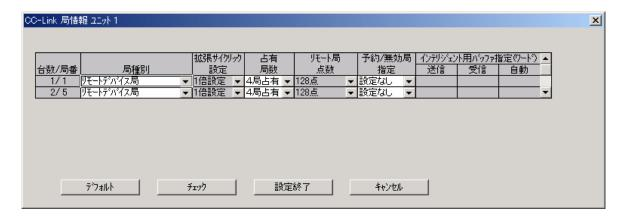
In the station type, select [Remote device station]. In the number of occupied stations, select [4-station occupied]. In the reserve/invalid-station assignment, select [No setting].
