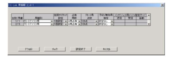
Select "Remote Device Station" in the **Station Type** field, select "4" in the **Occupied Stations** field, and select "None" in the **Reserved/Invalid Stations** field.
