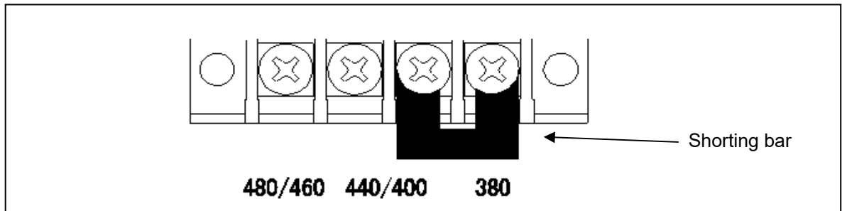
Figure 3-14 If the nominal voltage is 380VAC
